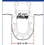
The Genesis Cyclone can generate a minimum trench width of 32.5" or 40", depending on model.
